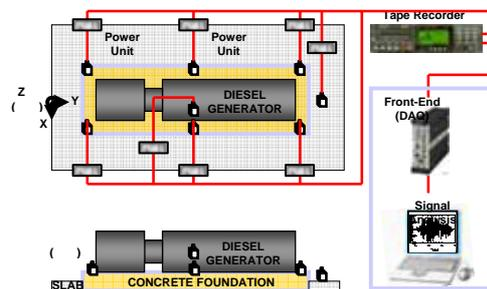
Fig. 3. Schematic Diagram of Measurement System
