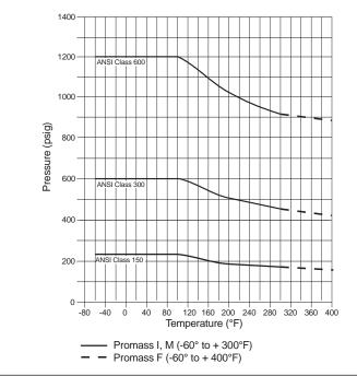
Maximum process pressure for titanium flanges is temperature independent: 150 lb ANSI: 230 psig 300 lb ANSI: 600 psig 600 lb ANSI: 1200 psig
