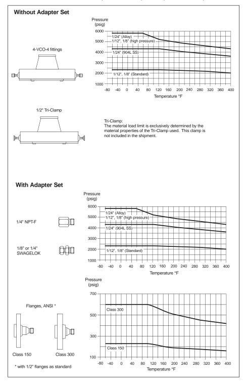
Material load curves for Promass A process connections
