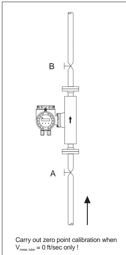
Zero point calibration and shut-off valves
