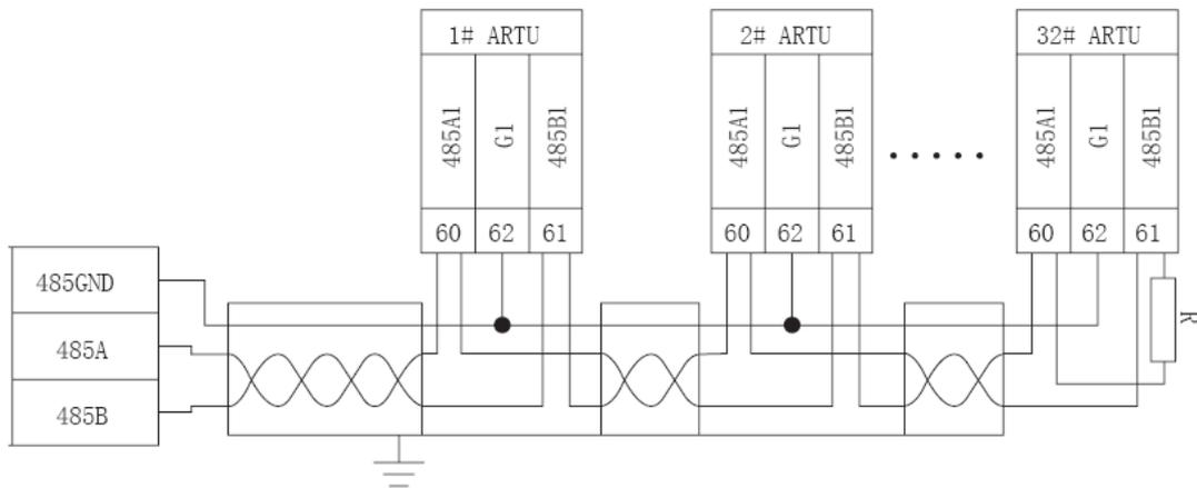
Note: When in a network, there are several PZ-K32, the connectors A and B of last PZ-K32 have to parallel one terminal R (120ohm~10kohm) to assure suitable communication resistance. According to the wiring, the terminal R is different.
