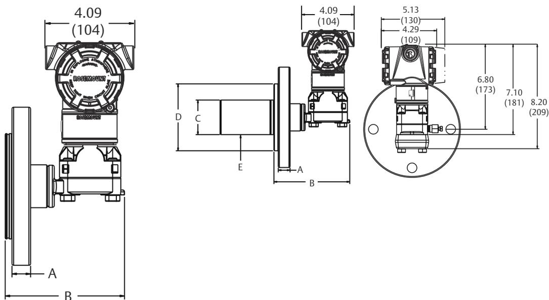
E. 2-, 4-, or 6-in. extension (only available with 3- and 4-in., DN80, and DN100 flange configurations)
