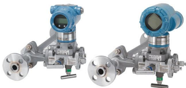
Rosemount 3051CFP Integral Orifice Flow Meters enable highly accurate flow measurement in small line sizes. Integral Orifice Flow Meters use precision honed pipe section for increased accuracy and self-centering plate design to prevent alignment errors that magnify measurement inaccuracies in small line sizes.
