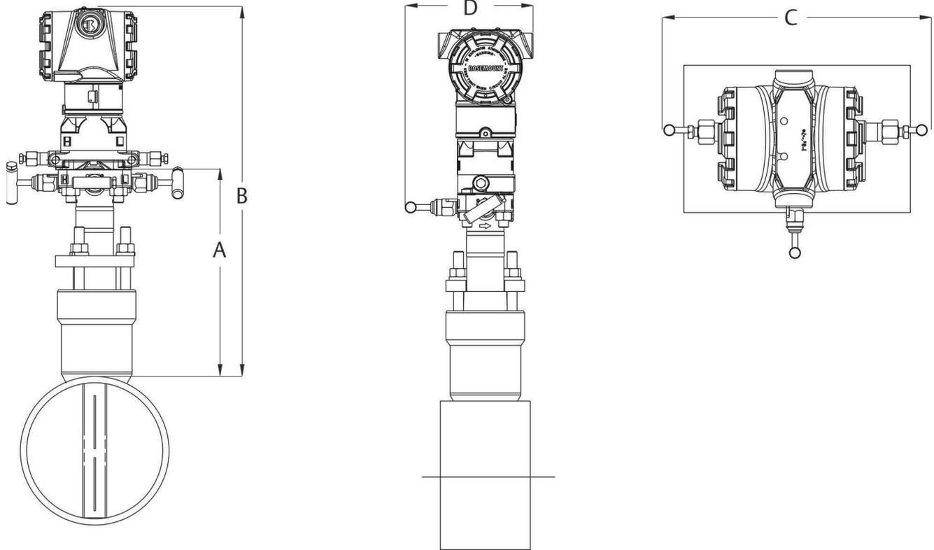
**Table 27: Rosemount 3051CFA Pak-Lok Annubar Flow meter Dimensional Data (Maximum Dimensions)**
