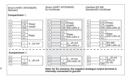
Terminal assignment: \*jumper selection in preparation HART = registered trademark of the HART Communication Foundation INTENSOR= registered trademark of Endress+Hauser
