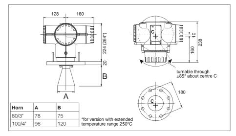
Dimensions in mm of Micropilot FMR 130 (with flange type DN 100 PN 16)
