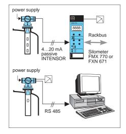
Measuring system Micropilot FMR 130: Remote operation is possible with handheld terminal or Commubox with laptop
