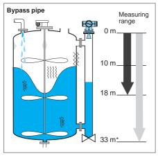
Typical measuring range as a function of antenna and application
