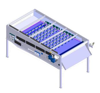
The DEWA BTN Gravity Belt Thickener is a fully enclosed system, designed to increase the dry solid concentration of the feed sludge considerably. Enclosed construction enables odor containment within the unit, simplifying odor extraction by the ventilation pipe located on the top of the cover. This advanced and sophisticated design concept creates a clean and odor-free environment.
