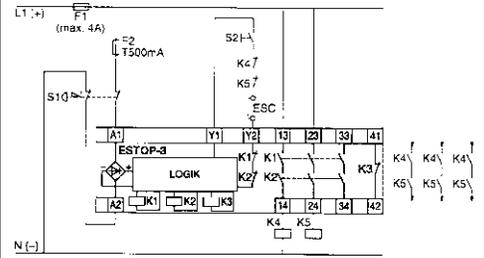
Emergency-stop button with one NC contact / 1 channel
