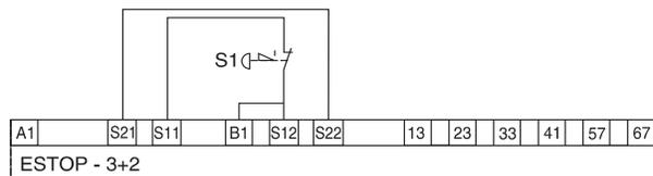
S1: Emergency stop button with 1 N/C contact
