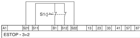
S1: Emergency stop button with 2 contacts (a short-circuit between the 2 inputs is not detected)
