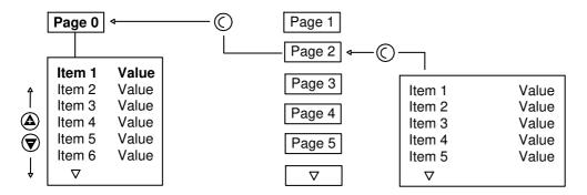
Press and hold RESET for two seconds at any time to immediately exit menu mode and return to the normal operational mode display. Any value or option adjustment that has not been confirmed and entered into memory will be abandoned and the original setting maintained.
