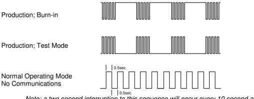
Note: a two second interruption to this sequence will occur every 10 second as the S1 broadcasts output data on the RS485 communications port.
