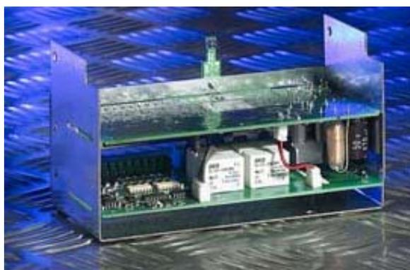
XPC Di8R4: 8 x digital input, 4 x relay outputs
