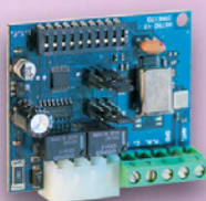
ASTRO 43/2R - plug in radio receiver card. 2 channels
