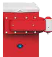
9897L ALA.180. This device allows for the beam to swing away (rotate) in the direction of the collision in case a vehicle crashes against it and is so designed to prevent the structural components of BAYT 980 automatic barrier and the beam from getting damaged. The device can be supplied factory-fitted or be fitted to installations of BAYT 980 already existing. Limits of application: beam 6.400 mm max. or 4.200 mm max. with a fence
