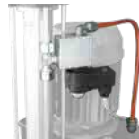
9873L Blackout device. 24 Vdc solenoid valve. In case of power failure, it is possible to raise the beam by hand. It is always to be combined with the voltage stabilizer code 9321L for the installation to work properly. The device is factory-fitted
