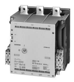
CONTACTOR SIZE 14, 3-POLE AC-3, 335KW, 400/380V (690V) AUXILIARY CONTACTS 44 (4NO+4NC) AC OPERATION AC 200 TO 240V 50/60HZ
