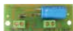
AJ01410 adapter to use limit switches kit AJ01400 with F4PLUS and BA100 boards
