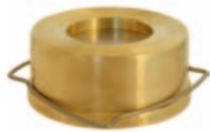
RK 71 with spiral centering PN 6 to PN 16, body material hot-pressed brass, valve disc of austenitic steel
