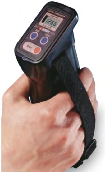
The SBS-2002 is lightweight, durable and easy to use, making it suitable for use in all industrial environments. Simply insert the nozzle into the battery and depress the finger pump which draws a few drops of sulfuric acid ( $H_2SO_4$ ) through the tube. Within three seconds the measured refractive index is converted into a temperature-compensated specific gravity reading and then both the specific gravity and temperature are displayed.
