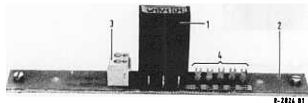
Fig. 3 Internal reference junction compensation (width 3E, E = 5.08 mm)
