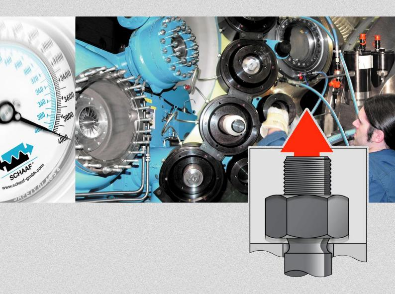
**SSV** and **HM** – Axial bolt tensioning without torquing!
