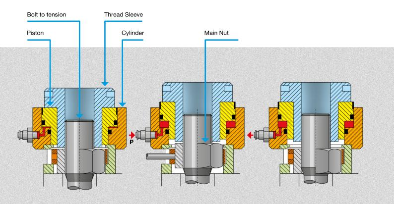
Bolt Tensioners can be removed from the bolt connection after pre-tensioning: in comparison, Hydraulic Nuts remain on the bolt or component connection.
