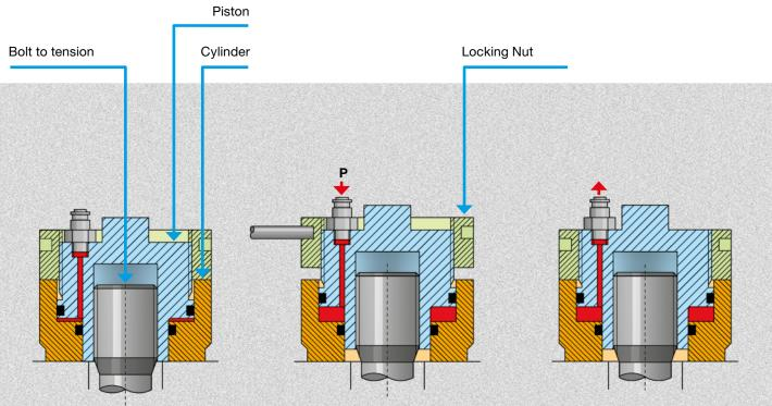
Hydraulic Nuts do not require a thread projection as Bolt Tensioners do and, therefore, can be used in older constructions to replace conventional torque wrenched bolt connections. For large bolt connections in particular, this eases work and increases the safety of the tension force. Compared with Bolt Tensioners, Hydraulic Nuts enable quicker changing times for connections that need tightening and loosening on a regular basis. This speeds up checking load forces.
