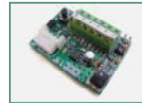
P111408 - SCS WIE Circuit board for direct connection of wiegand accessories (such as SELETTO, COMPAS SLIM, etc) to the control units QSC D MA, LIBRA C MA, LIBRA C MV, LIBRA C LX, VENERE D, LEO D MA, LEO MV, RIGEL 5 and ALTAIR P.
