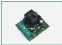
D111761 - ME BT 12/24 Vac electric lock board for BT operators.
