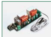
P111376 - SCS 1 Serial connection board for QSC D MA, LIBRA C MA, LIBRA C MV, LIBRA C LX, VENERE D, LEO D MA, LEO MV, RIGEL 5 and ALTAIR P.
