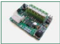
P111408 - SCS WIE Circuit board for direct connection of wiegand accessories (such as SELETTO, COMPAS SLIM, etc) to the control units
