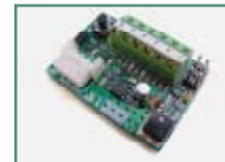
P111408 - SCS WIE Circuit board for direct connection of wiegand accessories (such as SELETTTO, COMPAS SLIM, etc) to the control units QSC D MA, LIBRA C MA, LIBRA C MV, LIBRA C LX, VENERE D, LEO D MA, LEO MV, RIGEL 5 and ALTAIR P.
