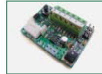
P111408 - SCS WIE Circuit board for direct connection of wiegand accessories (such as SELETTO, COMPAS SLIM, etc) to the control units QSC D MA, LIBRA C MA, LIBRA C MV, LIBRA C LX, VENERE D, LEO D MA, LEO MV, RIGEL 5 and ALTAIR P.
