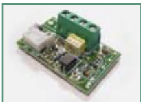
P111376 - SCS 1 Serial connection board for QSC D MA, LIBRA C MA, LIBRA C MV, LIBRA C LX, VENERE D, LEO D MA, LEO MV, RIGEL 5 and ALTAIR P.
