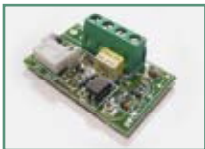
P111376 - SCS 1 Serial connection board for QSC D MA, LIBRA C MA, LIBRA C MV, LIBRA C LX, VENERE D, LEO D MA, LEO MV, RIGEL 5 and ALTAIR P.
