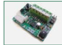
P125005 - BT BAT Thanks to the back-up batteries and battery charger, the BT BAT kit guarantees low voltage operation of the leaf in the event of power failure (LIBRA C MA, LIBRA C LX, HYDRA R).
