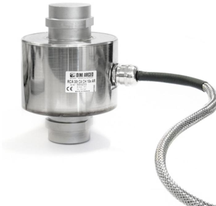
Analogue version of compression load cells, ideal for CE-M approved weighbridges, tanks, silos, etc. Manufactured in STAINLESS STEEL, IP68 protection, 4000 divisions, fitted with "rodent proof" armoured cable.
