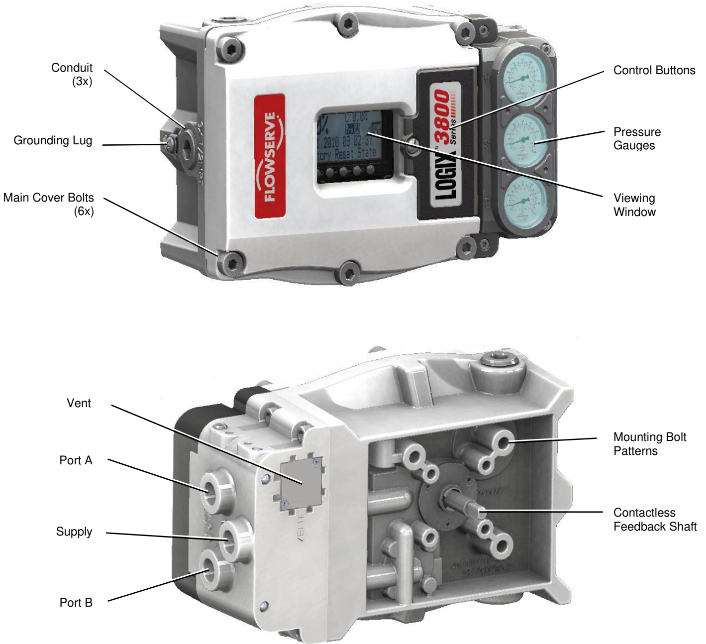
Figure 1: Logix 3800 External Positioner Features (EX and SS)
