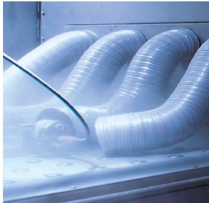
Design and build a prototype, abuse it until it fails, analyze the failure, improve the design, test it again. That's what Highly-Accelerated Life Time (HALT) Testing is all about. In-house HALT testing assures that potential design weaknesses are identified and subsequently eliminated.
