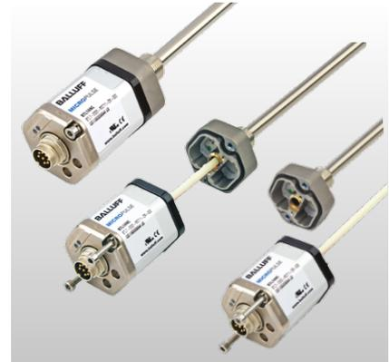
Micropulse BTL7 in-cylinder rod style sensors with the Rapid Replacement Module (RRM) option reduce potential downtime by allowing super quick and easy replacement of the electronics and sensing element without the need to break the hydraulic seal. No need to de-pressurize the system, and no worries about oil spillage. Spare modules can be pre-configured offline, saving time during replacement and setting equipment back into service faster.
