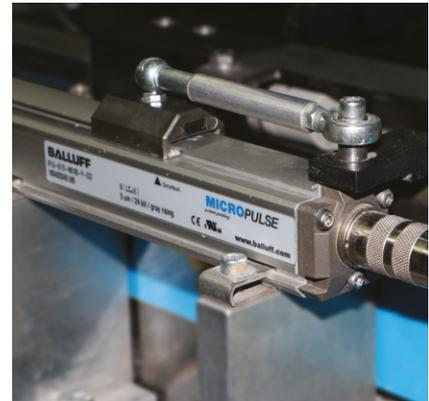
Extruded aluminum profile and low profile form factors are ideal for external-mount machine position monitoring applications. Patented Autotuning technology allows free-floating magnet operation, while the proprietary hard-anodized coating ensures nearly frictionless operation of the rod-operated sliding type magnet.
