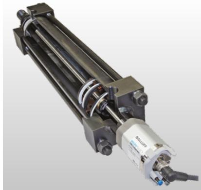
Micropulse rod style linear position sensors represent the new standard for hydraulic cylinder position sensing. The high-pressure stainless steel sensor probe is optimized to withstand hydraulic pressure up to 600 bar. Micropulse rod-style sensors are available in a variety of form factors and are built to order in lengths up to 7620 mm.
