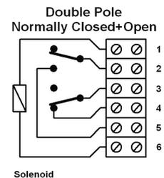
Switches are shown in their normal system operating position after a manual or remote reset has been performed
