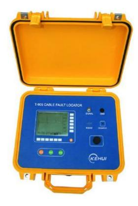
Combines Time Domain Reflectometer (TDR), Impulse Current Method (ICM) and Secondary Impulse method (SIM) for fault detection, T-905 Power Cable Fault Locator is designed to locate all kinds of power cable faults, such as open circuit, short circuit, low insulation, high insulation and flashover faults for electric power industries.
