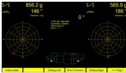
Unbalance values display at the end of the measurement.
