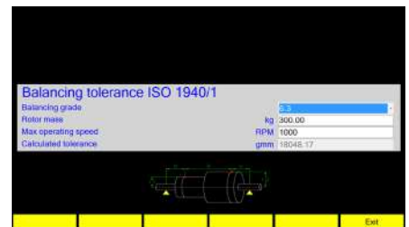
Unbalance tolerance calculation according to ISO 21940 standard.
