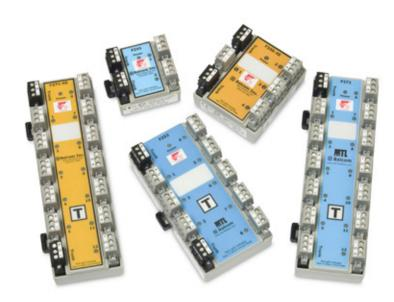
Megablocks are DIN-rail mounted passive hubs for Foundation™ fieldbus networks. They connect several field devices to the network trunk cable and provide short circuit protection to the segment. Megablocks minimize hand wiring and allow individual devices to be added to and removed from the segment without disrupting network communication.
