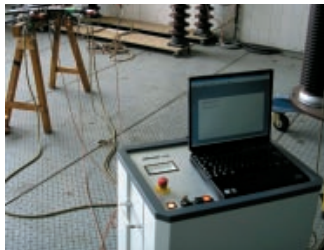
Fig. 8: CDS measurement in a high voltage laboratory
