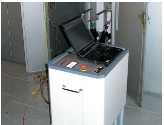
Fig. 7: CDS setup during a field measurement
