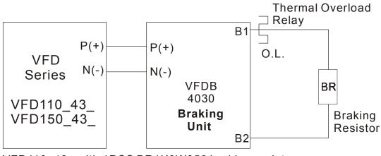
VFD110\_43\_ with 1PCS BR1K0W050 braking resistor VFD150\_43\_ with 1PCS BR1K5W040 braking resistor
