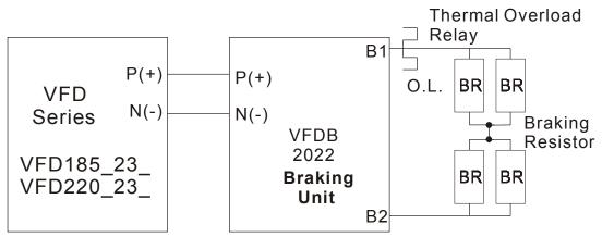
VFD185\_23\_ with two BR sets in series, which 2PCS BR1K2W008 braking resistors in parallel for each BR set.
