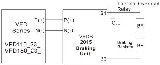
VFD110\_23\_with 2PCS BR1K2W6P8 braking resistors in series VFD150\_23\_with 2PCS BR1K5W005 braking resistors in series
