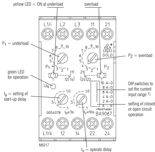
**1) Attention:** The required measuring range must be selected by putting the relevant DIP-switch to left position. All other range selector DIP-switches are in right position.
