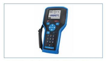
The protective rubber boot provides added protection in the field.
