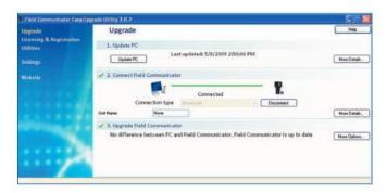
The Easy Upgrade Utility allows you to transfer system software, DDs, and HART device configurations between the 475 Field Communicator and a PC.
