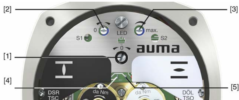
Figure 35: View on control unit when switch compartment is open
