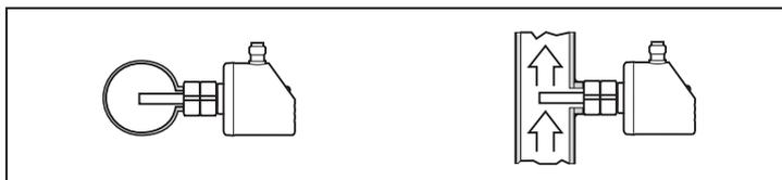
Fig. 2: Recommended mounting position
