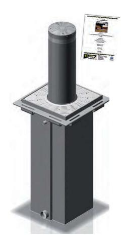
Pit is made of steel sheet alloy, thickness e 2mm and frame to be welled in. Main frame is ductile casted iron GS400, treated with cataphoresis.
