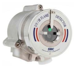
electromagnetic spectrum. The signals from both sensors are analyzed for frequency, intensity and duration. Simultaneous detection of radiant energy in both the UV and IR sensors triggers an alarm signal.
