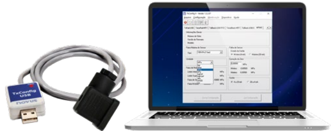
Configuration via the TxConfig DIN43650 interface and the free TxConfig II software
