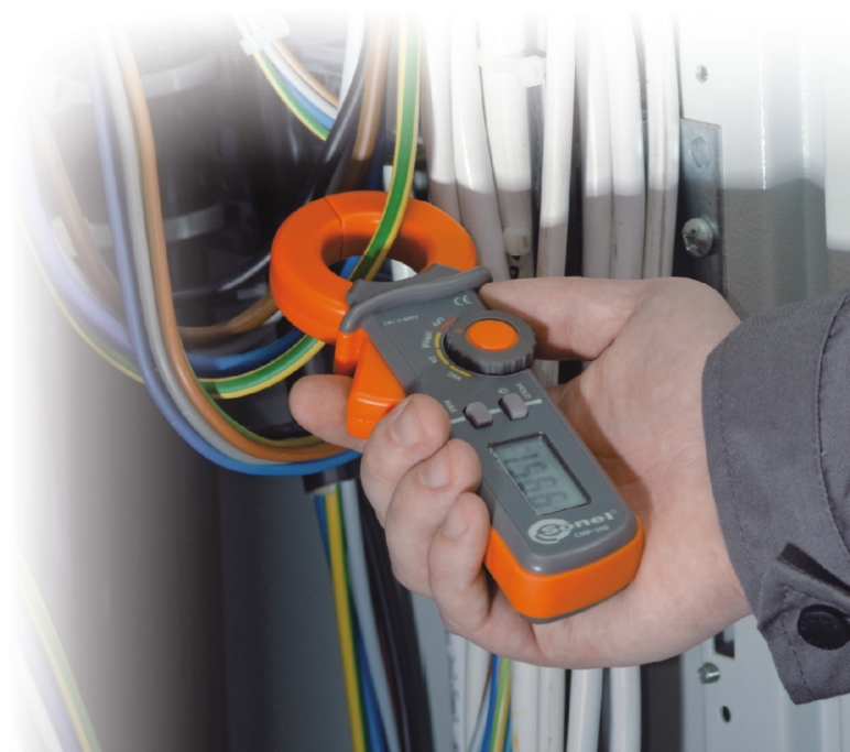
Rys. 2. Load current measurements.
