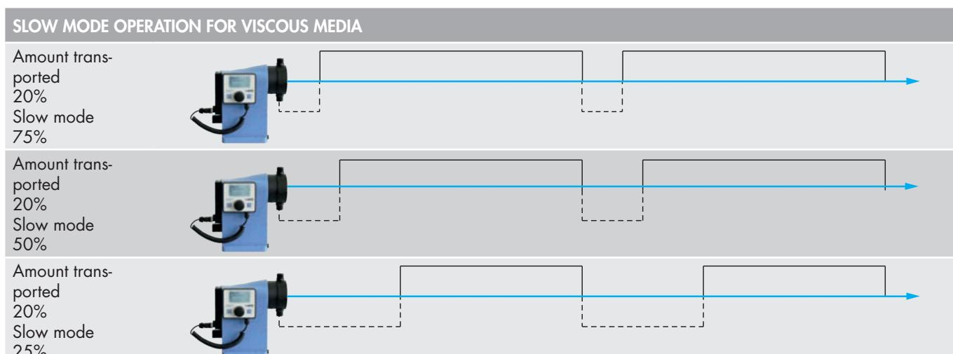
Pressure stroke      Time      Suction stroke
