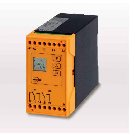
prompted through the programming sequence by parameter symbols on the LCD display. After entering the password, the user can adjust the high and low voltage limit points, phase imbalance margin (as a percentage of voltage measuring range), and relay energise / de-energise delay times upto 24.9 seconds. The instrument can thus be configured exactly per the application requirements.
