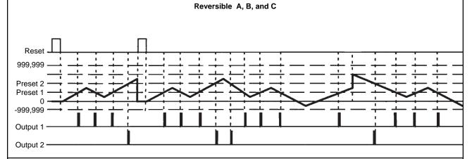
**Output Mode L** Present value increments and decrements within displayable range. Output 1 is ON whenever present value is less than or equal to preset 1; Output 2 is ON whenever present value is greater than or equal to preset 2.
