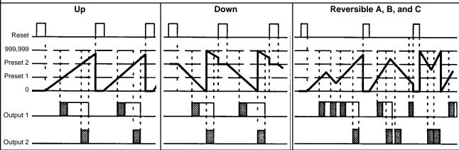
**Output Mode P** Present value display does not change during one-shot time period, but reset start status returns as soon as preset count is reached. Outputs are one-shot and operate repeatedly. Output 1 latches ON at preset 1, and goes OFF after expiration of the one-shot period for Output 2. One-shot time periods for Output 1 and 2 are independent.
