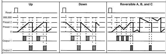
**Output Mode K** Present value runs continuously. Output 1 latches ON at preset 1, and goes OFF after expiration of the one-shot period for Output 2. One-shot time periods for Output 1 and 2 are independent.
