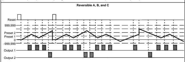
**Output Mode D** Present value increments and decrements within displayable range. Output 1 is ON whenever present value is equal to preset 1; Output 2 is ON whenever present value is equal to preset 2.
