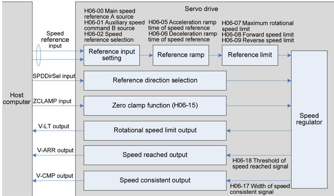
The main use procedure of the speed control mode is as follows:
