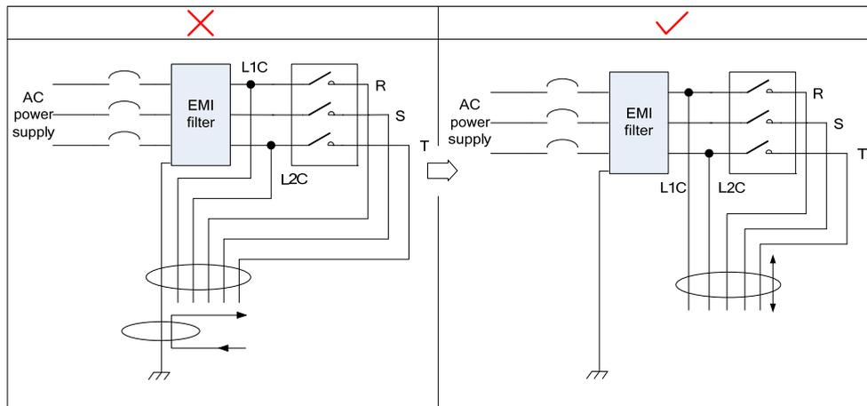
3) Use a separate grounding cable as short and thick as possible for the EMI filter. Do not share the same grounding cable with other grounding devices.
