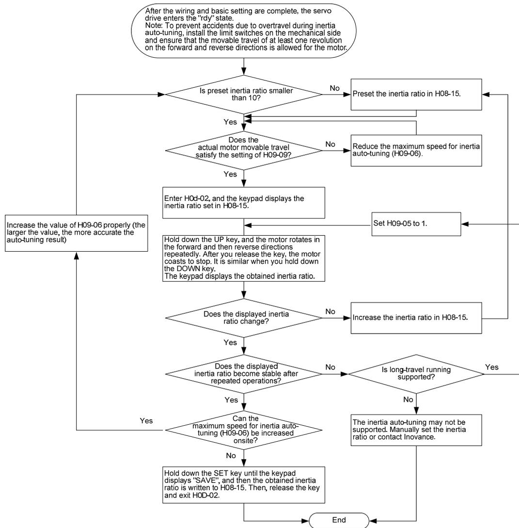
When H08-15 = 1 (default value), the actual speed may not reach the reference due to too small inertia ratio, and the auto-tuning will fail. In this case, you need to set H08-15. It is recommended that H08-15 be set to 5 initially and then increased gradually so that the auto-tuning can be performed successfully.
