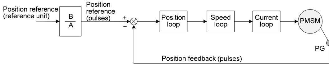
When H05-02 is 0 and the motor is connected to the load through the reduction gear, assume that the reduction ratio between the motor shaft and the load mechanical side is  $n/m$  (the load shaft rotates  $n$  revolutions when the motor shaft rotates  $m$  revolutions), and the formula of calculating the electronic gear ratio is as follows:
