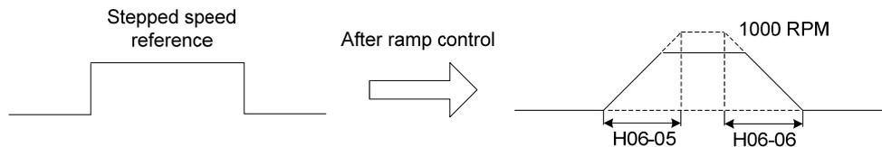
H06-05 specifies the time for the speed reference to accelerate from zero to 1000 RPM.
