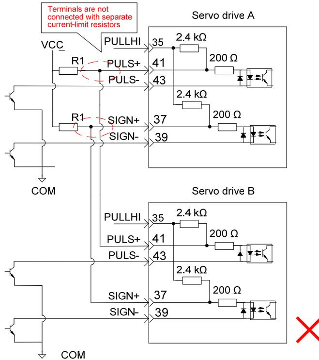
High-speed reference pulse and symbol signals at the host controller can only be output to the servo drive via differential drive output.
