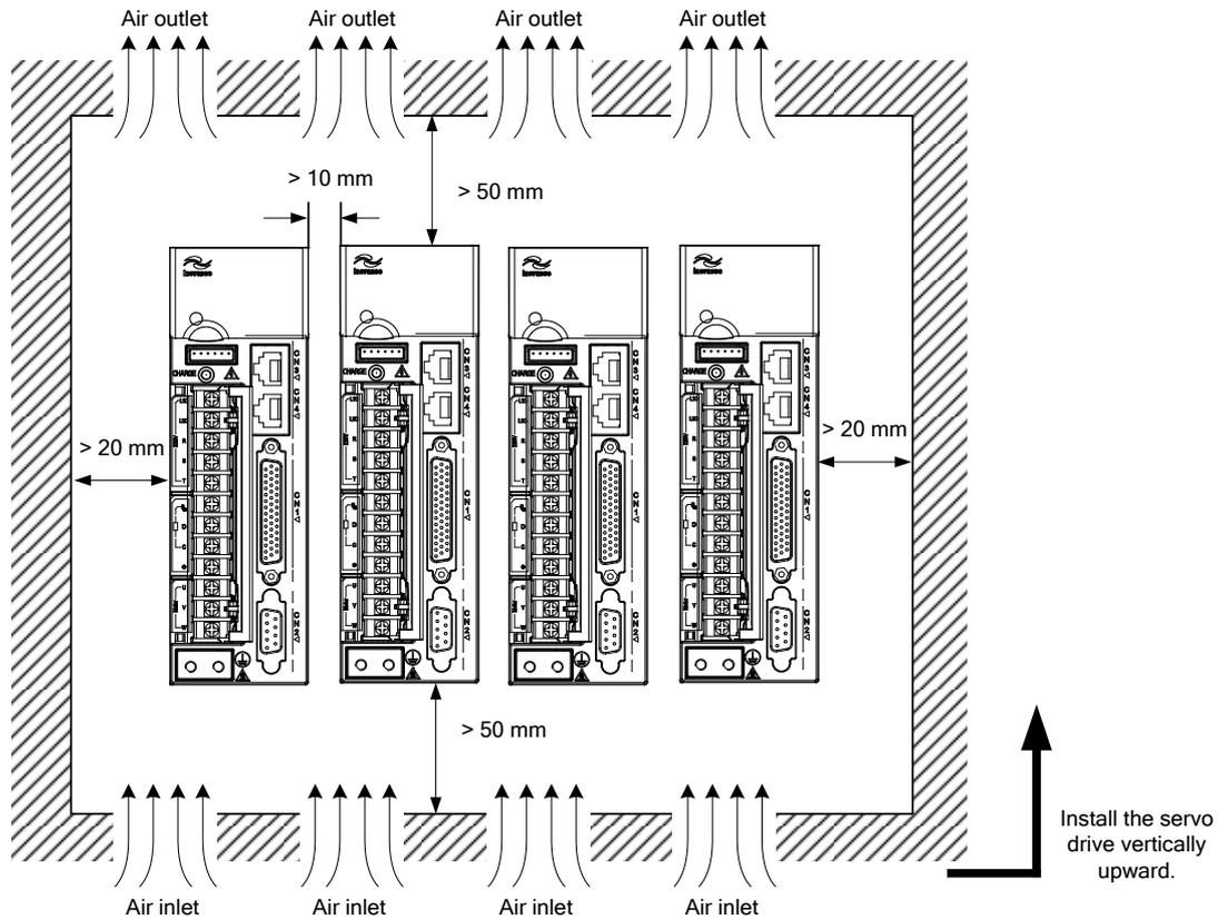
Install the servo drive vertical to the wall, making its front panel faces outward.
