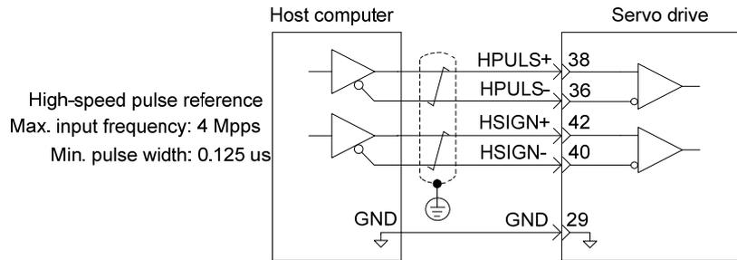
Make sure the differential input is 5 V. Otherwise, input pulses of the servo drive are unstable, which will cause:
