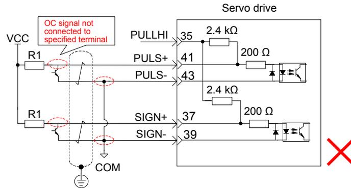
Multiple terminals share the same current-limiting resistor, resulting in that pulses are inaccurately received.
