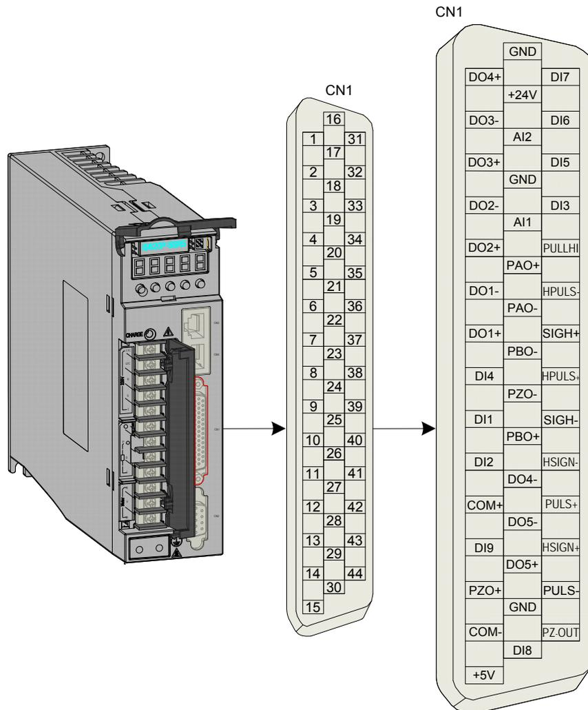
CN1 terminal: Plastic housing the connector plug: DB25P (TELE-DATA COM), black housing; Core: HDB44P (TELE-DATA COM)
