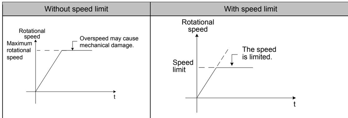
When the rotational speed is limited, the DO terminal outputs the signal described in the following table.
