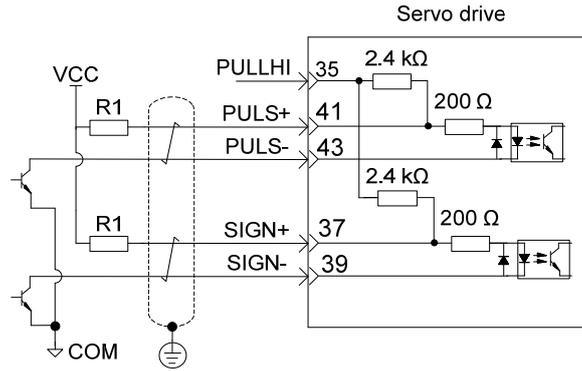
Value of resistor R1 shall satisfy the following formula:  $\frac{V_{CC}-1.5}{R1+200} = 10\text{mA}$
