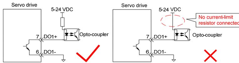
The maximum allowable voltage and current of the optocoupler output circuit inside the servo drive are as below:
