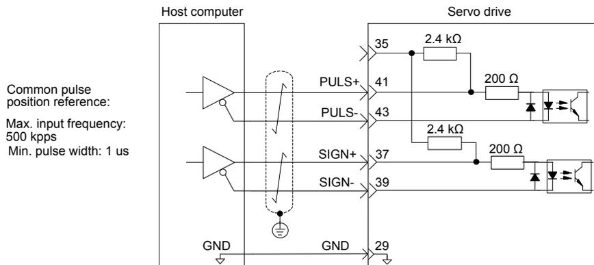
Make sure “ $2.8\text{ V} \leq (\text{H level}) - (\text{L level}) \leq 3.7\text{ V}$ ”. Otherwise, input pulses of the servo drive are unstable, which will cause:
