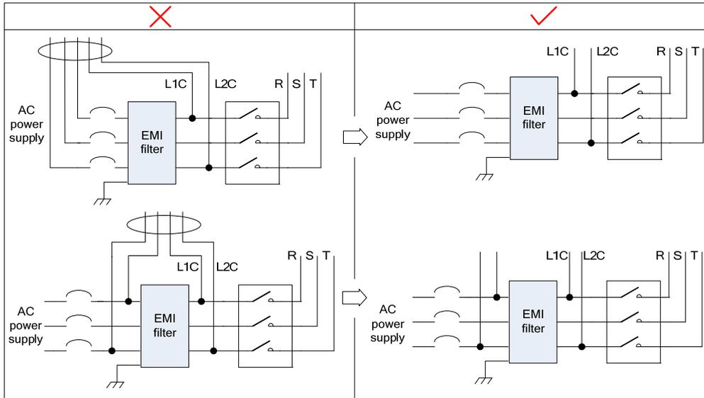
2) Separate the grounding cable and output power supply line of the EMI filter.
