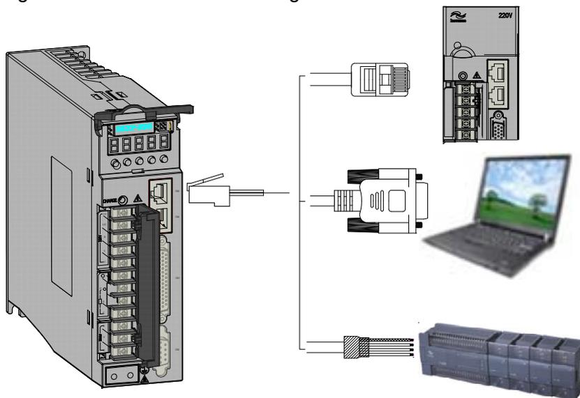
CN3 and CN4 are two same communication signal terminals connected in parallel. Do not
