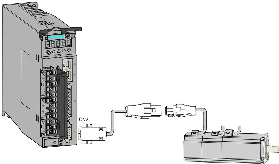
Table 3-8 Connectors of encoder cables at servo drive end
