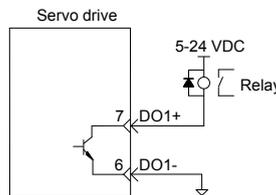
Wrong connection 1: Current-limiting resistor is not connected, resulting in burnout of terminals
