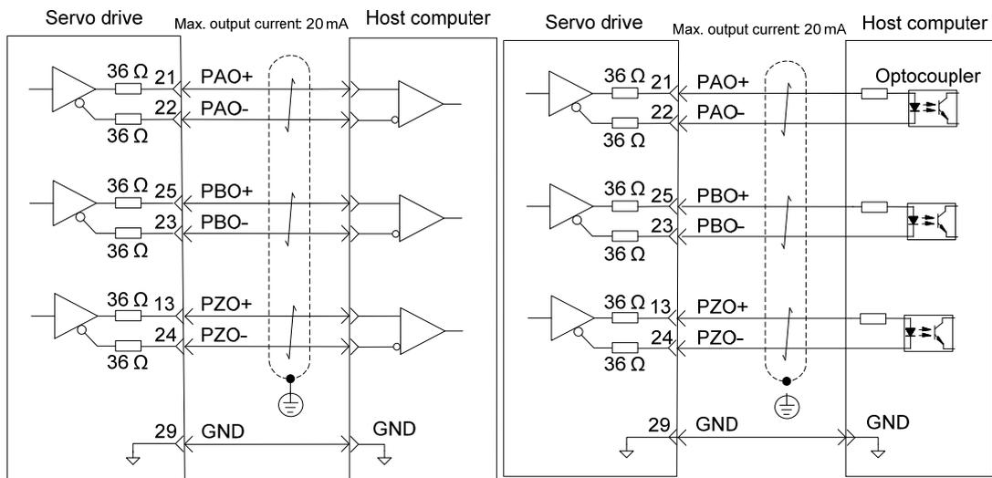
Encoder phase Z output circuit outputs OC signals. Normally, the encoder phase Z output circuit provides feedback signals to the host controller. The circuit and the host controller together form a closed-loop position control system. An optocoupler circuit, relay circuit, or bus receiver circuit shall be used in the host controller to receive feedback signals.
