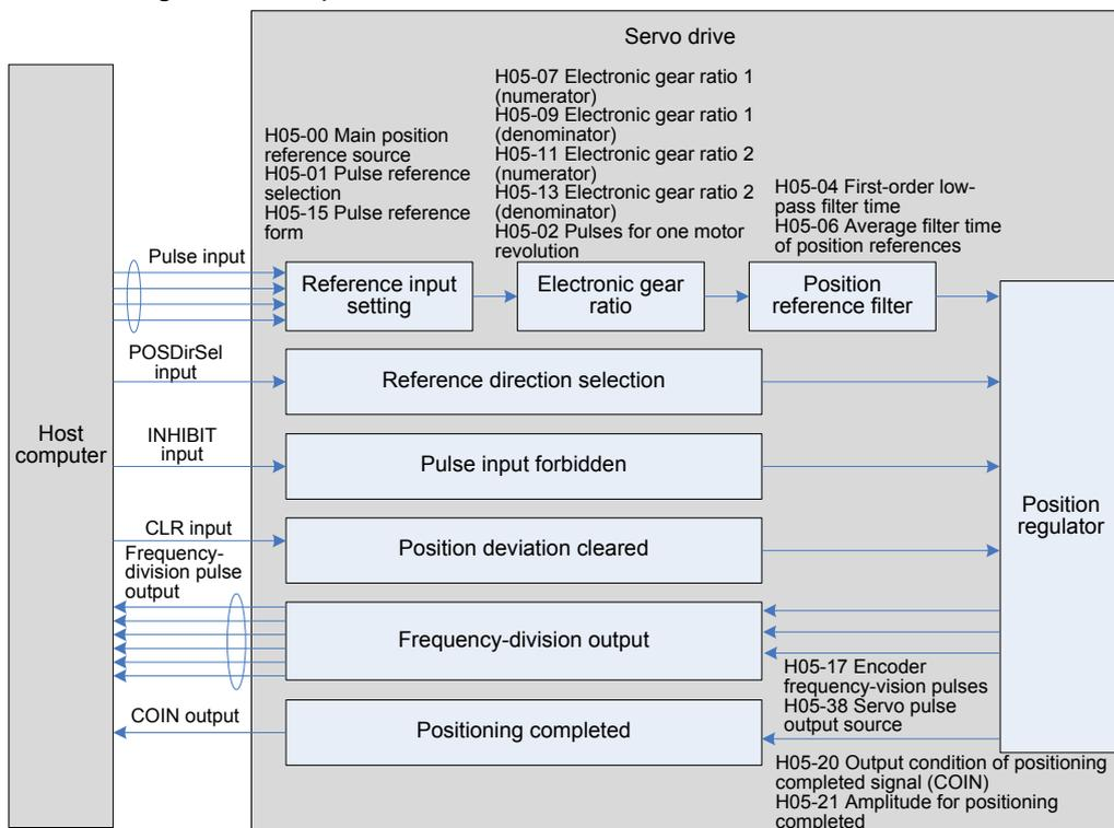
The position control mode is the most common mode of the servo drive. The main use procedure is as follows:
