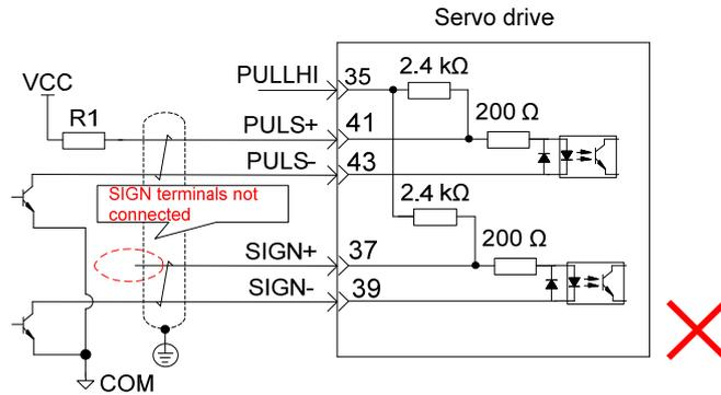
Wrong connection 4: Terminals are inaccurately connected, resulting in burnout of terminals.
