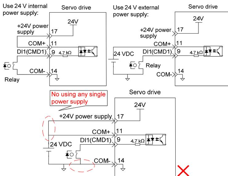
b) When output signal of the upper device is OC output:
