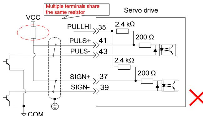
Wrong connection 3: SIGN terminals are not connected, resulting in that these two terminals receive no pulses.
