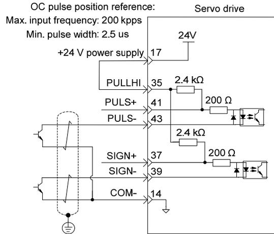
Wrong connection: Pin 14 (COM-) is not connected, which cannot form a closed-loop circuit.
