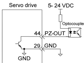
The 5 V ground of the host controller must be connected to GND terminal of the servo drive to reduce noise interference. The maximum allowable voltage and current of the optocoupler output circuit inside the servo drive are as below:
