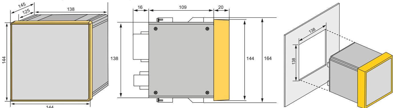
A front-panel cutout of 138 mm x 138 mm is required for the device.
