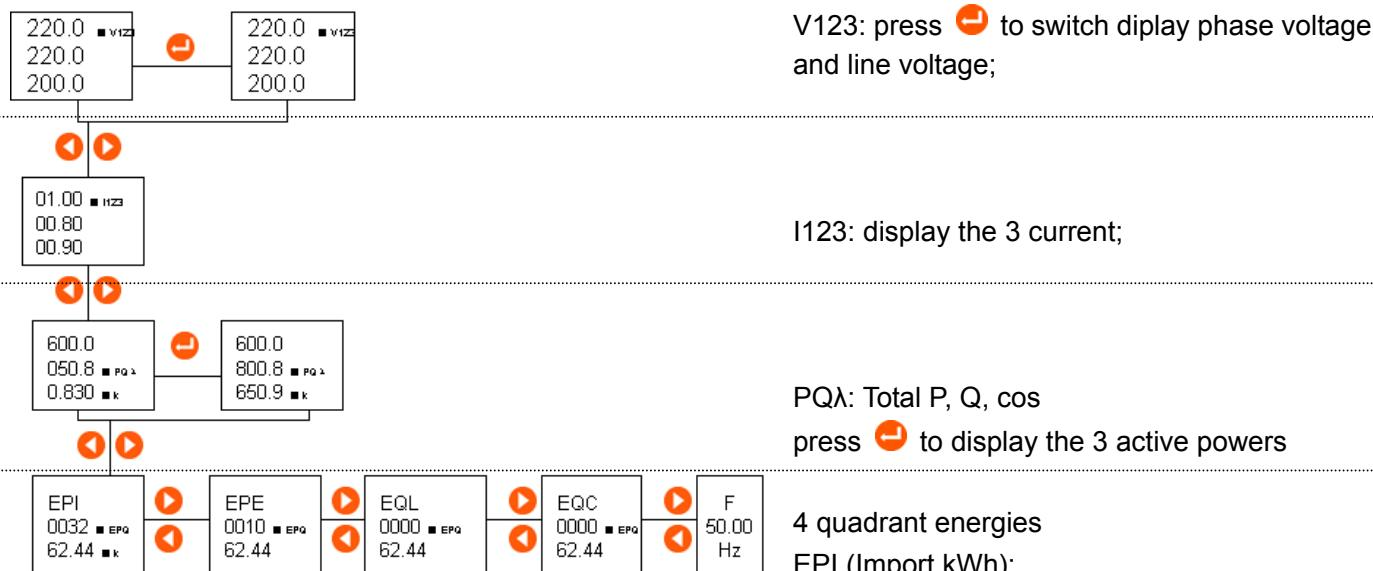
Press, keep and loosen to change the display.
