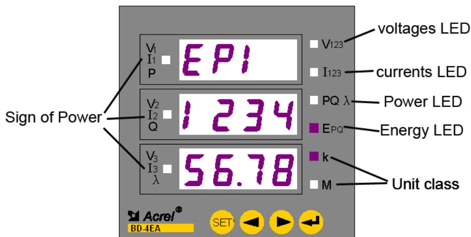
When the left LED is of power sign active, it indicates the P/Q/cos in this line is negative.
