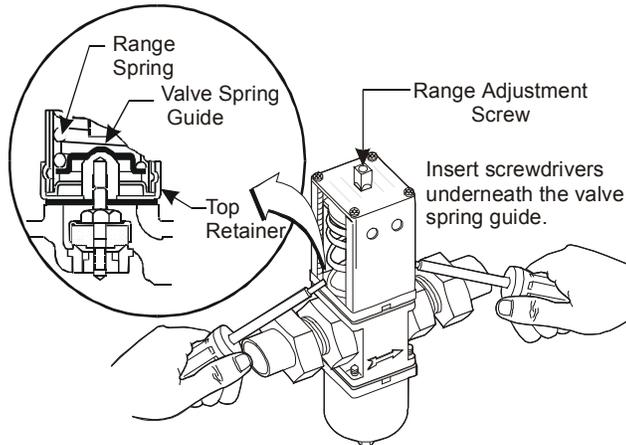
**Figure 2: Manual Flushing**
