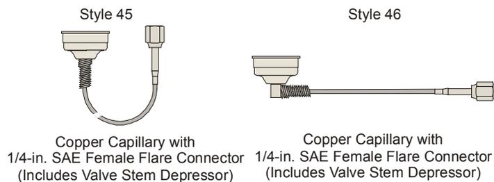
**Figure 3: Pressure Connection Styles V46\_connectors**
