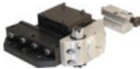
Worm gear slides for Heavy wall pipe
