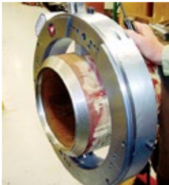
Weld ready after machining
