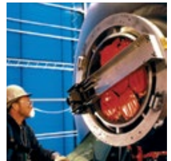
Optional Bridge Slide for Heavy Wall Pipe
