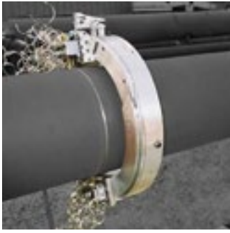
Simultaneous parting and beveling
