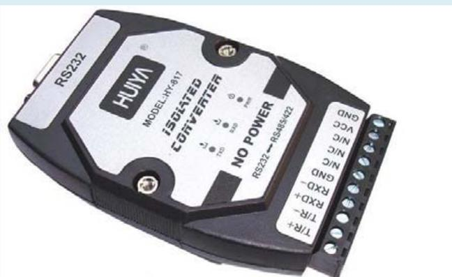
3. Protection class: RS485.RS422 interface with 600W lightning surge protection per wire
