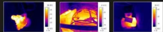
Working electrical devices cause heating. By comparing the thermal images taken by YRH250/600, the potential malfunction of the electrical devices can be found earlier.
