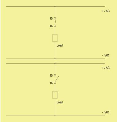
Contacts 15-16: Voltage free contact for Line and Load Fault detection.
