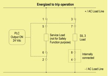
Contacts 1-5 and 2-6: closing of this contact can be used to monitor contacts 3 - 7.
