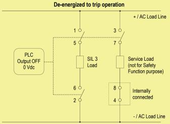
Contacts 1-5 and 2-6: the SIL 3 Safety Function is met when the relay is de-energized, contacts are open, SIL 3 load is de-energized.
