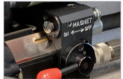
Protection against motor start-up when magnetic base is not activated
