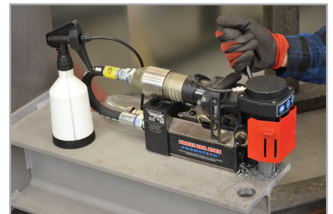
Through spindle cooling system
