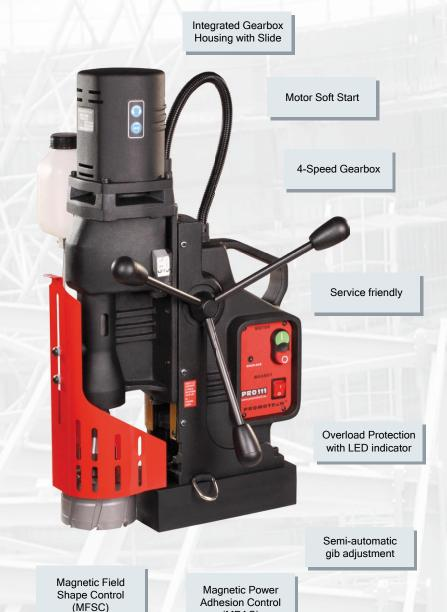
PRO 111 is equipped with electromagnetic base featuring magnetic field shape control system (MFSC) and magnetic power adhesion control module (MPAC), which detects adhesive force of electromagnetic base and protects both the machine and the operator from work on too thin workpieces.
