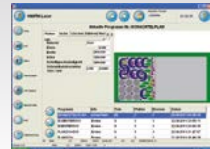
Contour nesting on grid remainder and separation of excess plate material (optional)
